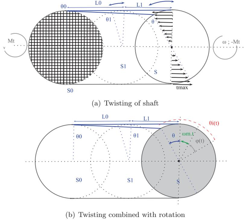
Figure 3: Shaft in twisting and in rotating
