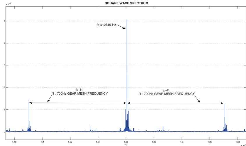
(b) Gear mesh frequency
