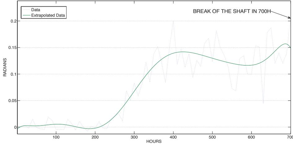
Figure 5: Standard-deviation of the instantaneous phase  $\theta_i(t)$
