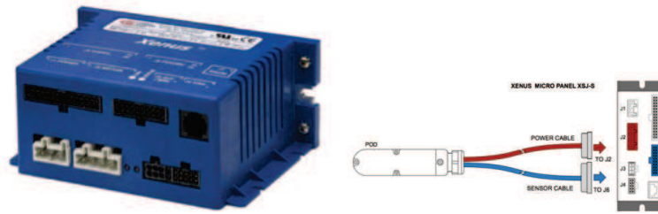
Figure 4: Variable-speed drive and its connections to the motor
