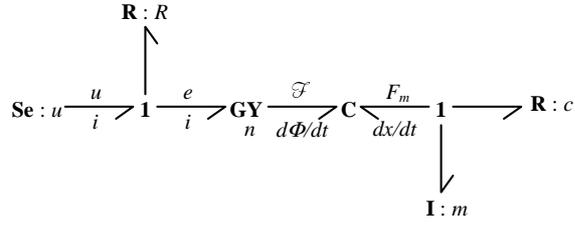
Fig. 3. Bond-Graph model of the actuator.
