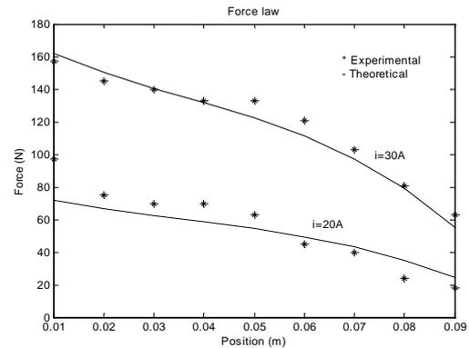
Fig. 2. Theoretical and experimental results of the force law.
