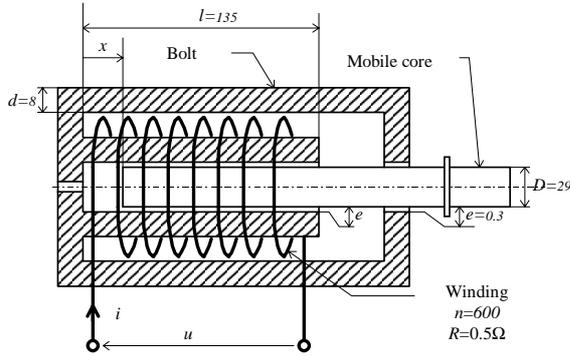
Fig. 1. Schematic diagram of the actuator.
