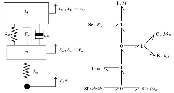
Fig. 5. Mechanical structure of an active suspension and its corresponding Bond-Graph model.
