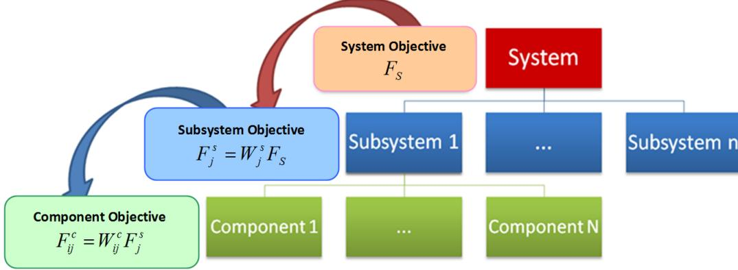
Figure 3: Allocation principle: The system Fault Frequency objective is allocated to subsystems and each subsystem Fault Frequency objective is allocated to components.
