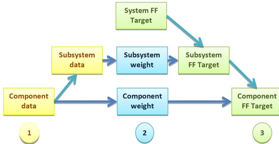
Figure 5: Computation procedure to allocate the system FF target to subsystems and then to the components.
