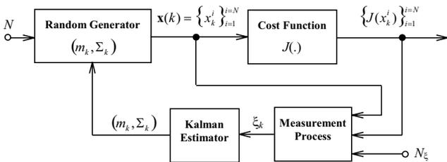
Fig. 1. Principle of the algorithm
